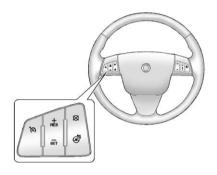
②: Press to turn the heated steering wheel on or off. A light on the button displays when the feature is turned on.
